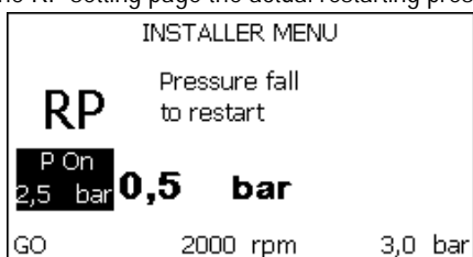
Figure 18.1: Setting the restart pressure (2)
